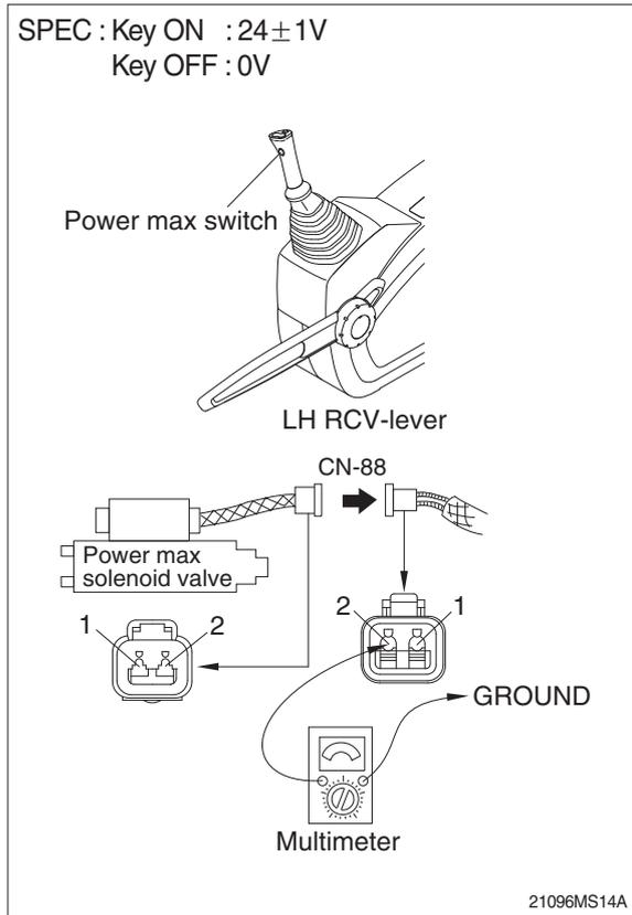
(2) **Test 18:** Check resistance of the solenoid valve between CN-88(1)-(2).
