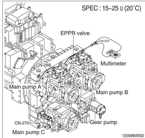
(2) **Test 2** : Check electric current at EPPR valve.
