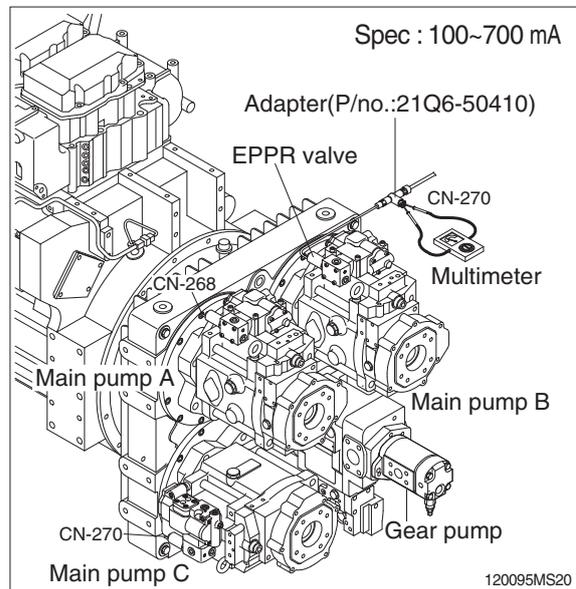
(3) **Test 3** : Check pressure at EPPR valve.
