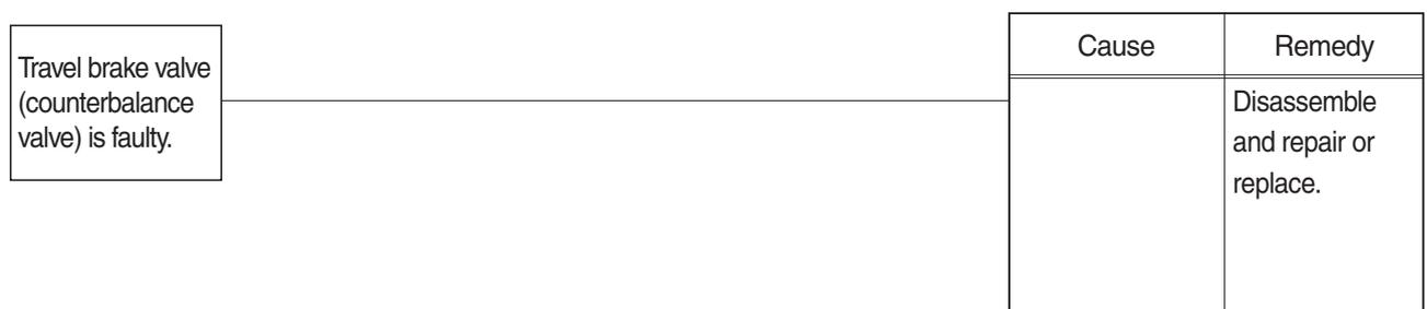
7) MACHINE MAKES A CURVED TRAVEL OR DOES NOT TRAVEL AT ALL WHEN TRAVEL AND ATTACHMENT OPERATIONS ARE EXECUTED AT THE SAME TIME
