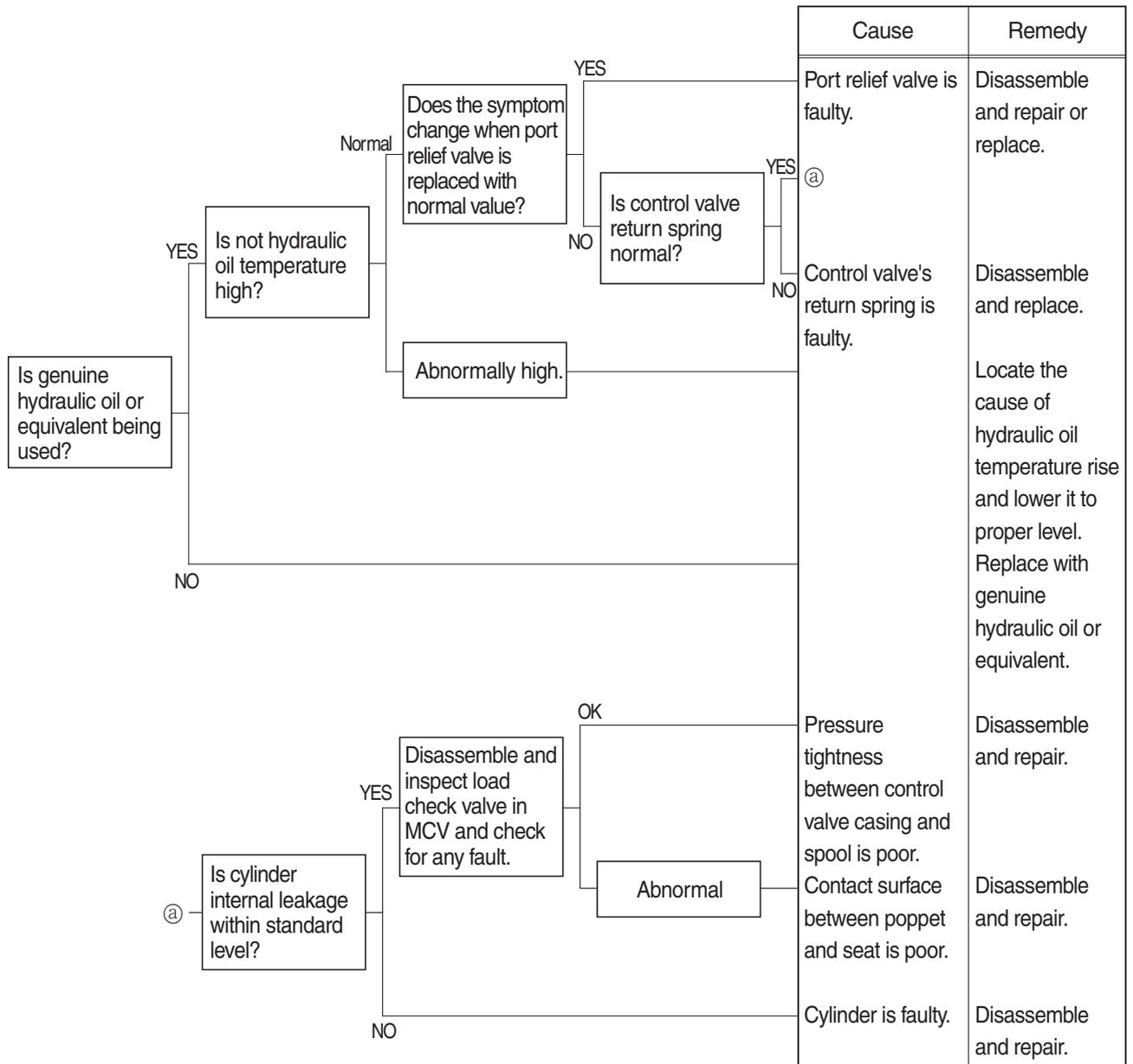
6) BOOM MAKES A SQUEAKING NOISE WHEN BOOM IS OPERATED
