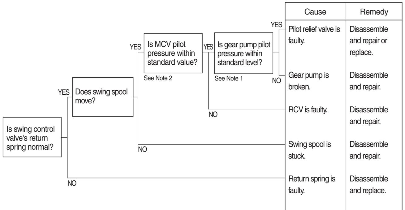
5) THE SWING UNIT DRIFTS WHEN THE MACHINE IS AT REST ON A SLOPE
